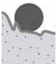
Large areas of the reinforcement are close or right at the concrete surface
